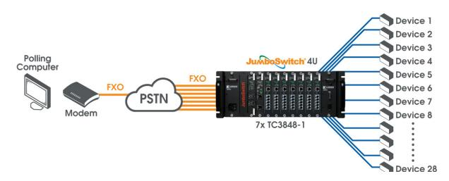
The TC3848-1 mounting is flexible: We can use a 1U rack to configure two cards and connect eight devices, all the way up to a 4U rack for up to seven cards connecting up to 28 devices.
