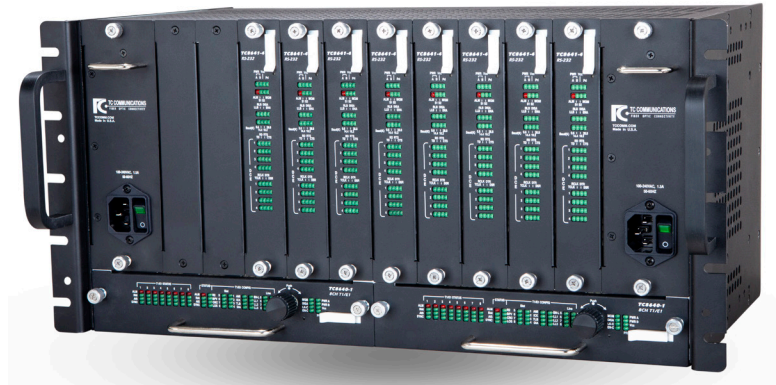
TC8641-4 in TCRM19E 5U Chassis with TC8640-1 T1/E1 Base Card (Front)
