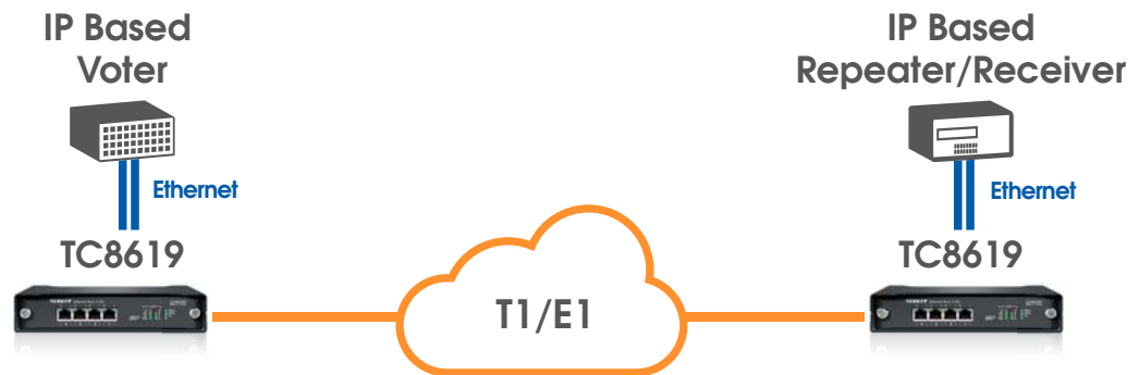
Figure 1-2 Typical Application using TC8619 Ethernet-over-T1/E1 Multiplexer
