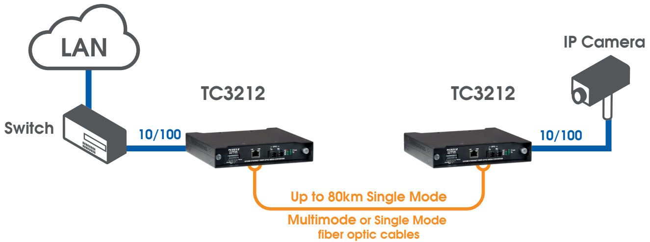
Typical Application Using TC3212 to Link an IP Camera Via Fiber
