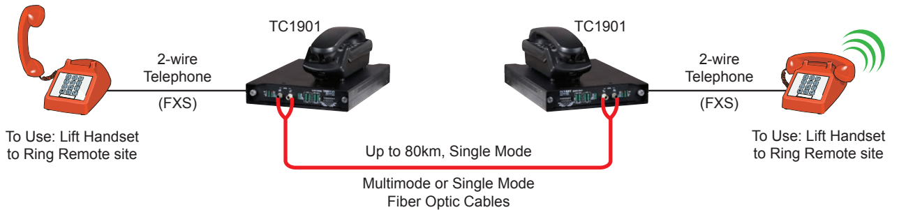
Typical Application Using TC1901s to Establish a "Hot Link" via Fiber Optic Cables
