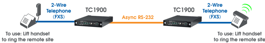
Typical application using TC1900s to establish a "Hot-Link" via RS-232
