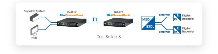
Once again, as soon as the system was connected it operated perfectly. There were no link alarms and the links were well within the required parameters. Multiple calls from the dispatcher were setup and again there was no increase in digital delay across the system.
