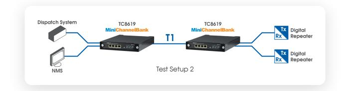
We placed multiple simultaneous voice calls through the dispatcher and the audio was crisp, clear and there was no increase in delay by using the T1 link.
