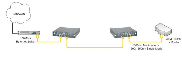
Typical applications using TC3004 Fiber Optic Mode Converter/Repeaters
