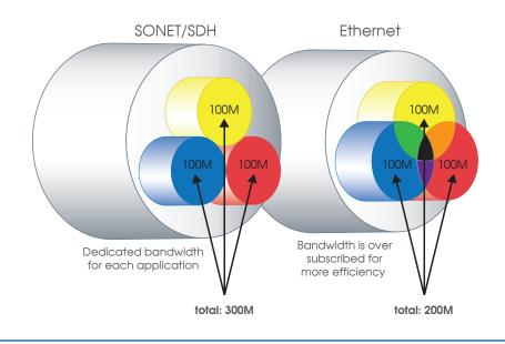
Figure 2: Bandwidth Efficiency Comparison
