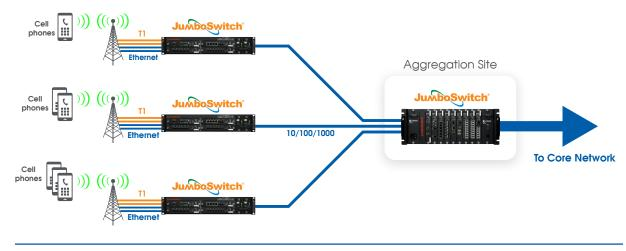
Figure 1: Ethernet Statistical Multiplexing Capability
