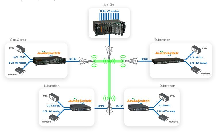
Power Utility uses JumboSwitch® MSEP Solution with Existing Ethernet Microwave Network to Replace Expiring Leased Lines
