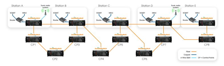
Metrolink and Centralized Train Controls (simplified). The actual network involves 6 stations and 22 control points (CPs).
