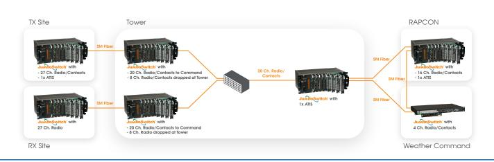
Above: JumboSwitch used to migrate radio communications for the airfield including command post weather, radar approach control (RAPCON) and the tower.
