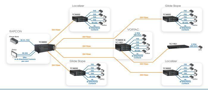
Above: TC8800 fiber optic multiplexer used to integrate Glide Slope and Localizer data as well as multi-site telephony for transport between multiple buildings, radar approach control (RAPCON), the airfield public branch exchange (PBX), and the automatic terminal information service (ATIS).
