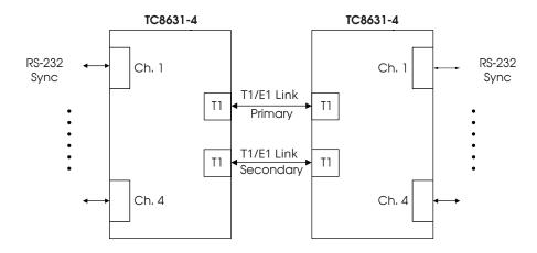
TC8631-4 Redundant Block Diagram
