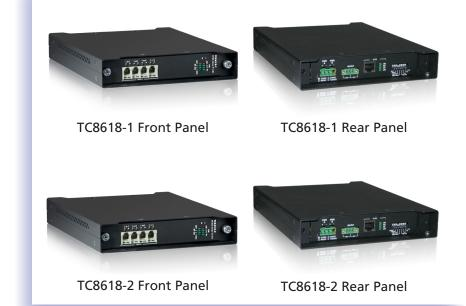
he TC8618 is a 4-channel Voice/Fax/Modem over T1/E1 Multiplexer that allows network managers the flexibility of leveraging T1/E1 circuits by adding low cost analog as needed. Dialing and paging between TC8618-1 (FXS) units is supported, providing customers flexibility for voice calls. The device is economical, simple to install and comes standard with built-in power redundancy.
