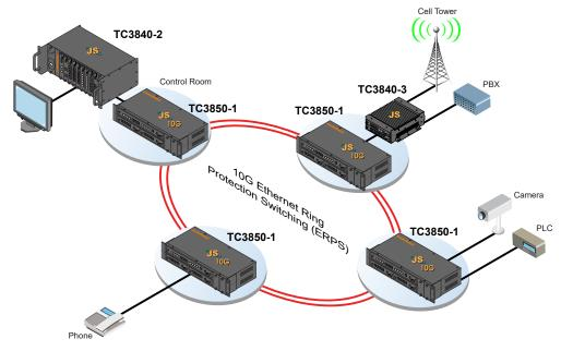
Typical Application Using the TC3850-1 to form an ERPS Network
