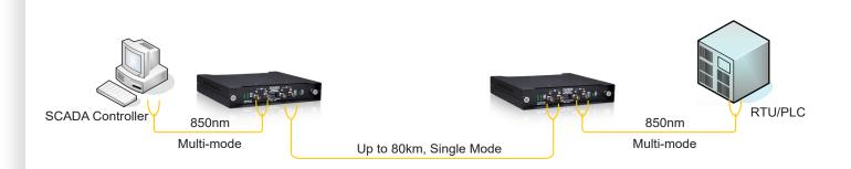
Typical Application Using TC3026 Fiber Optic Mode Converter
