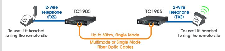
Typical Application Using TC1905s to Establish a "Hot Link" via One Fiber
