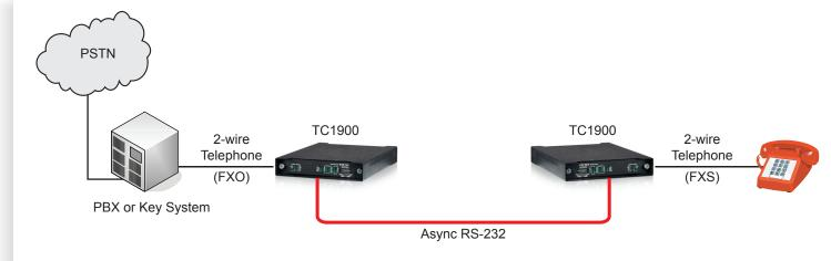
Typical Point-to-Point Application Using TC1900s to Extend Telephone via RS-232
