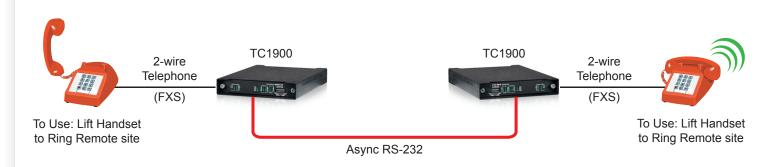
Typical Application Using TC1900s to Establish a "Hot Link" via RS-232
